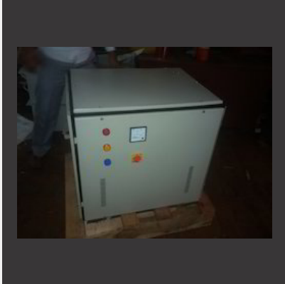
50 KVA Isolation Transformer
