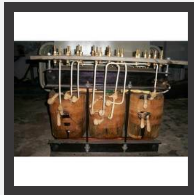
100 KVA Isolation Transformer
